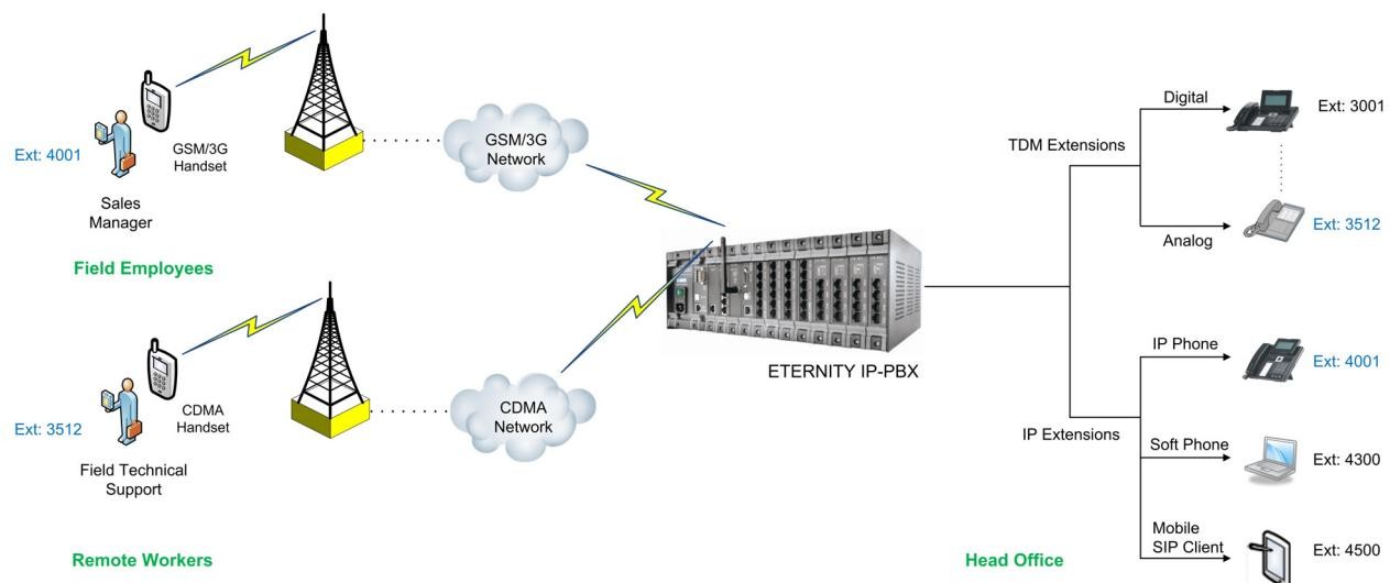
Here, as shown in the application diagram any GSM/3G/CDMA Mobile can work as an extension. Once programmed as Mobile Extension, users can make internal or trunk calls as well as attend desk calls from their mobile phone. While doing so, mobile phone users can access most of the system features in a similar way to other extensions of the PBX.
